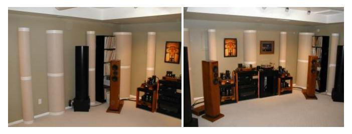
Accurately placing and rotating the traps makes a significant difference. I was surprised at how sensitive both placement and rotation are. Also it is quite important to place the traps so that there is accurate left to right symmetry. Use lots of traps and get real anal about how they are placed and you will love what these things will do for your system.
