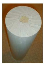
6. The next step is to wrap the trap with fabric. There are lots of ways to do this. With a little practice and experimentation you will be able to refine a technique that result in a smooth nice looking covering. What worked well for me was to stretch the fabric along one edge and staple on the top and bottom. Then
